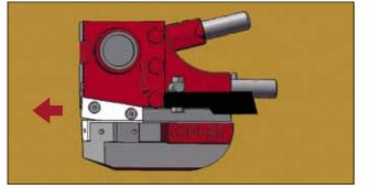
Loosen the two screws on the top blade (hexagon socket WAF 4)
