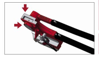
Alternatively, a grease nipple may be installed on the rear of the shears body. If there is one, use it as the lubrication point.
