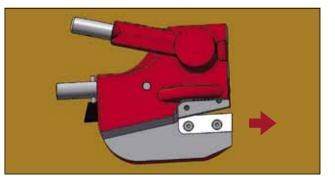
Loosen the two screws on the bottom blade (hexagon socket WAF 4)
