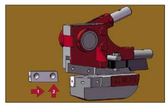
Secure the blade with the two blade screws. Tighten the blade screws to 11 Nm  $\pm$  0.5 Nm.
