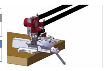
Use the round stop for cutting circular cuts or circular blanks.
