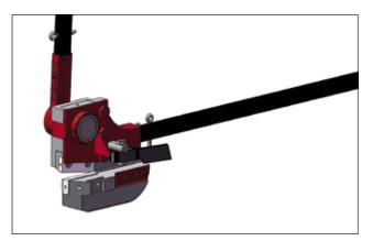
The blades are inclined towards each other, so that you can insert all material cross sections (that the shears can cut) up to the point where they touch the blades.
